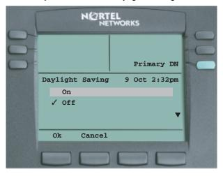
The "\( \sigma\)" in front of the time zone indicates your current selection (that is, Daylight Savings disabled). Press **Ok** to turn off Daylight Savings or press **Cancel** to return to the Time menu.
